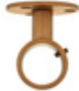
TFCS100MCMBK NEW 1" steel ceiling mount bracket 2" Dia ceiling plate, 2 1/4"H 2 1/8" drop (distance from ceiling to bottom of pole)
