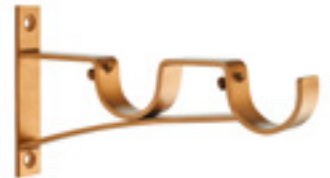
TFCS100LADBK NEW steel bracket, double 6" front and 3" back return, ¾"W x 3¾"L backplate
